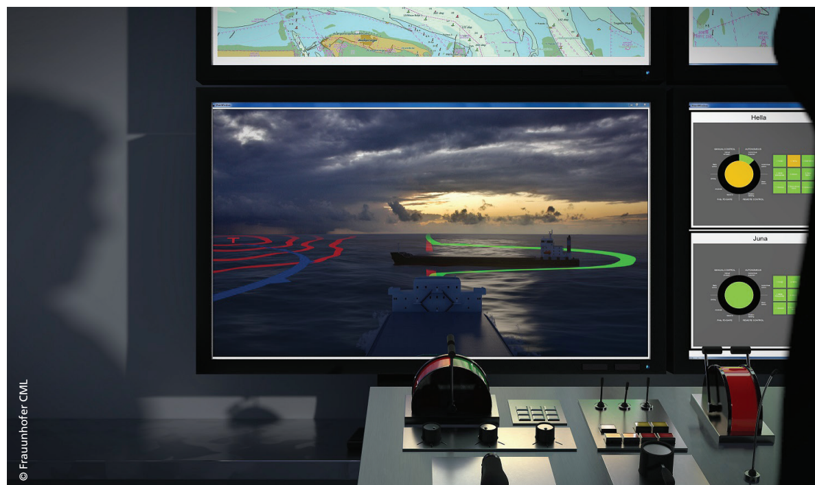
Evasive maneuver of an unmanned ship as visualized in the Shore Control Center SCC.
